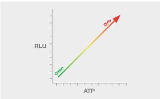
Higher RLUs indicate the presence of potential contaminants and recleaning may be required. Each facility must set its own acceptable levels to ensure proper cleaning and sanitation has taken place.
