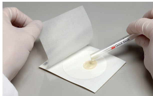
Inoculating 3M Petrifilm Plate using 3M Quick Swab
